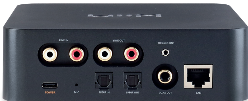
ABOVE: Powered via a 5V USB-C connection and with BT and Wi-Fi antennas inside the (plastic) box, the Pro Plus offers a wired Ethernet port, optical (192kHz/24-bit) and line inputs, coaxial and optical digital and analogue line outputs
